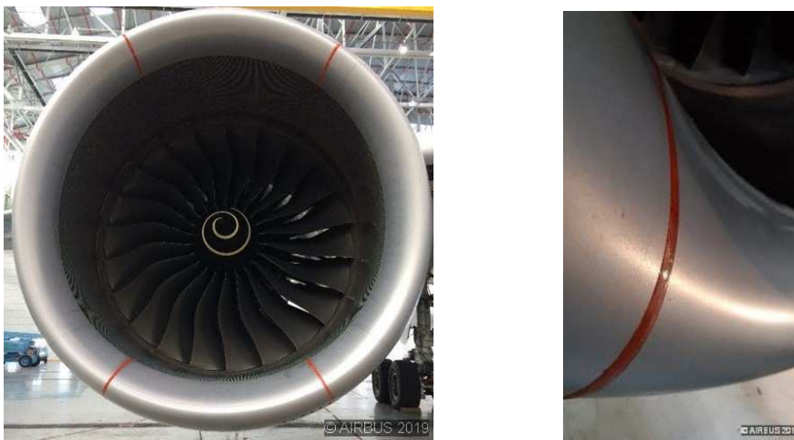
Fig.8: Pictures of the optical fibers integration on an aircraft engine inlet.
