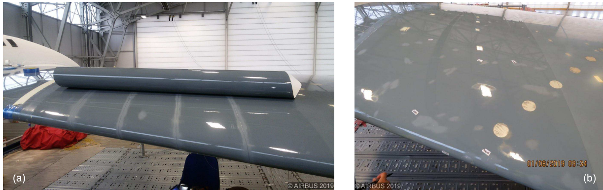
Fig. 3: a) Picture of the installation before upper sticker application, b) installation finalized
