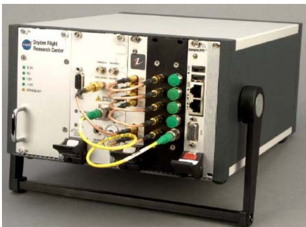
Figure 6-1: Ground-Based Four-Fiber Interrogation System and NESC CCM Testing.
